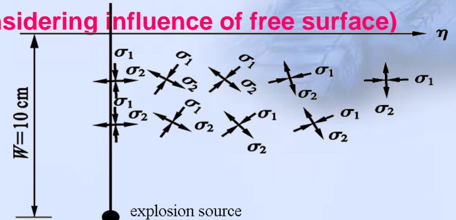
Direction of \sigma_1 and \sigma_2 when tensile stress \sigma_2 takes a maximum value
